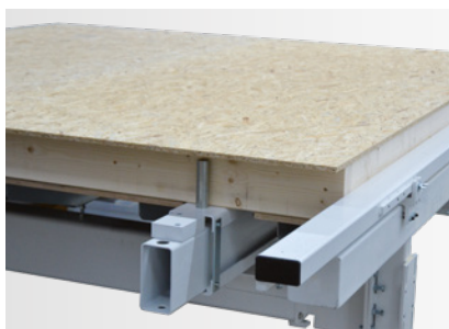
Elements can be aligned at the correct angle at the X stop.
