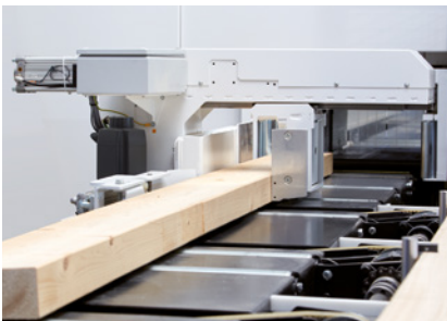
Beam carrier in the feed gripper
