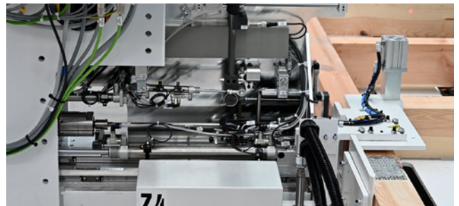
Screw unit for screwing frame works together.
