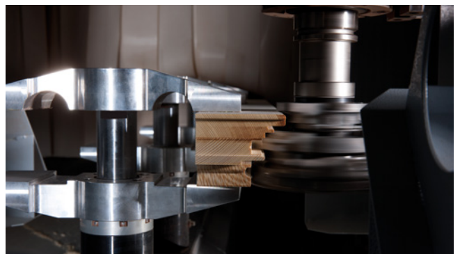
Liquid-cooled trimming spindles with vector control
